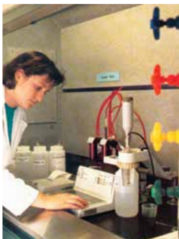
ABOVE: A lab technician with the Fuel Oil Testing unit of the American Bureau of Shipping tests a ship’s lubricating oil to be sure it doesn’t contain excessive acid. The maritime industry has invested heavily in environmental testing and compliance programs as regulatory demands have increased.
